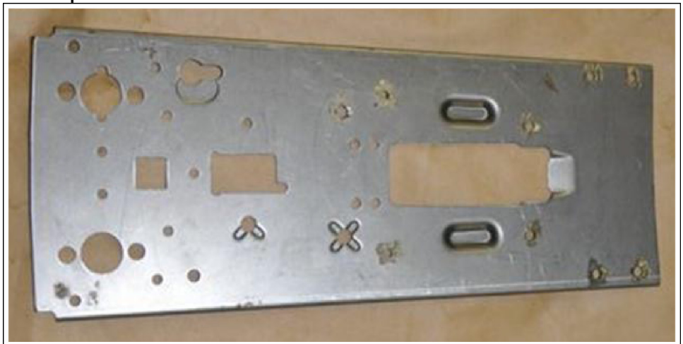
Figure 8: A Flat with All of the Required Holes Drilled but That Has Not Been Bent into Shape
